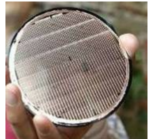
Micro-inductors fabricated on 4 inch Si wafer
